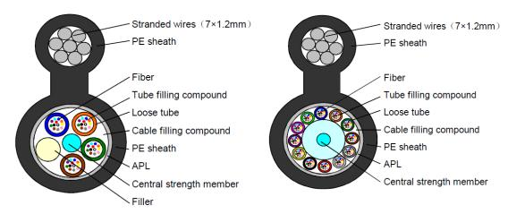
Note: Drawings are the 48 Fibers and 144 Fibers PE sheath cable as examples
